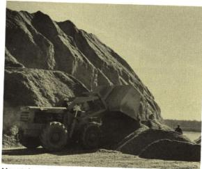
Mountains of wood chips from sawmill and plywood left-overs—once burned as waste—are now used for producing paper products.
