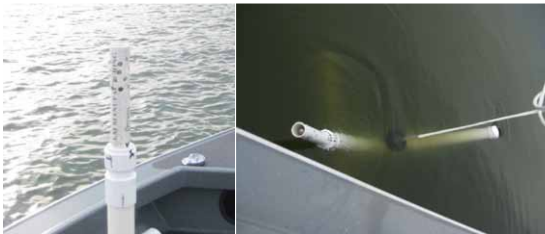
Figure 45. Probe casing and deployment for Bateman Island thermal data
