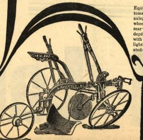
Equipped with the best bottoms made, adjustable front axle; dust-proof removable wheel boxes; adjustable rear wheel; easily set for any depth; works equally well with large or small horses; light draft and easily operited-a perfect plow.
