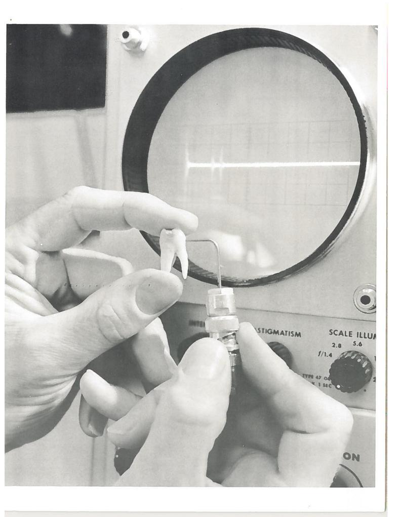
The idea of applying ultrasonics to biomedical uses came out of extensive work in the field of nondestructive testing techniques in nuclear energy research. The picture shows how an ultrasonic probe is used to detect early dental cavities without the use of X-rays. The research was initiated at Pacific Northwest Laboratory, sponsored by the Atomic Energy Commission. Further studies are being carried out under the sponsorship of the U.S. Public Health Service.
