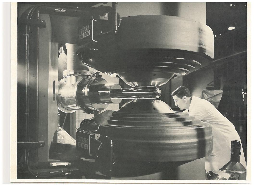
A polarized proton target being readied for use at Argonne
