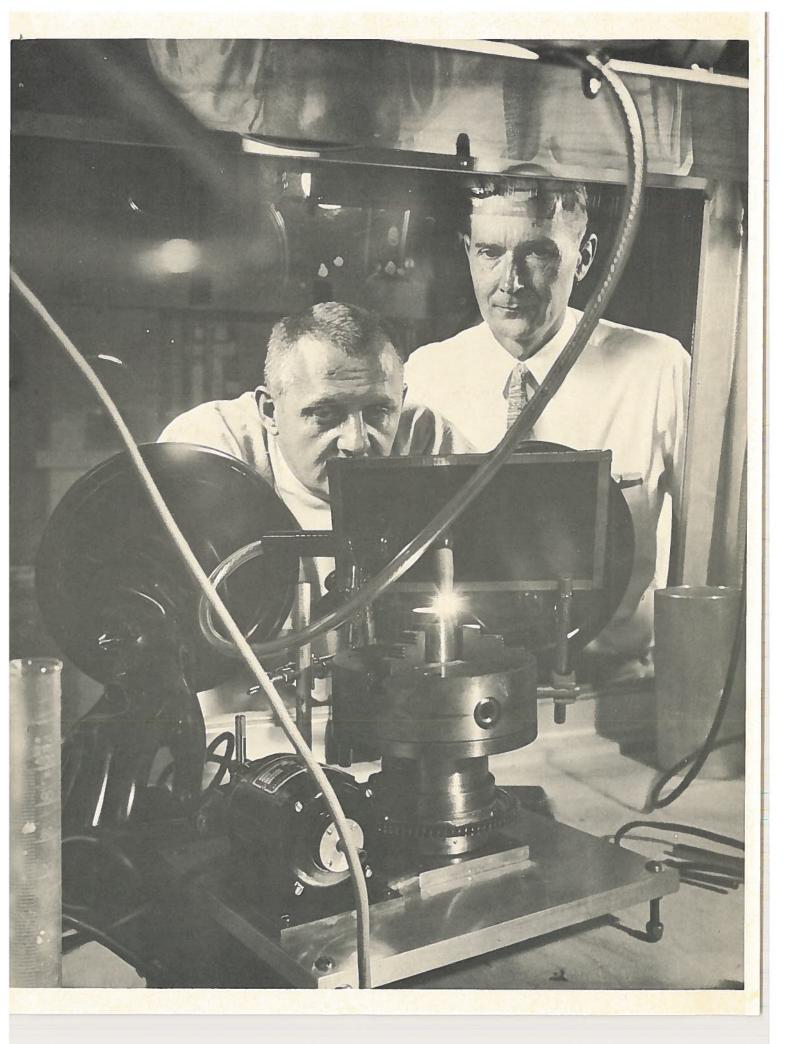
An end plug is welded to an irradiation capsule inside of a nitrogen filled glove box at Argonne National Laboratory. This capsule contains experimental plutonium fuel specimens which will be irradiated in an operating reactor. After the capsule has been irradiated, it will be disassembled in a heavily shielded cell and the specimens will be evaluated as potential fuel material for future reactors. No. 201-6572
