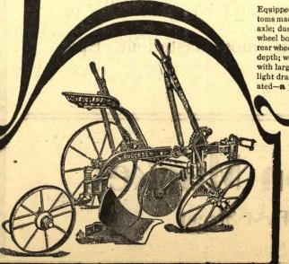
Equipped with the best bottoms made, adjustable front axle; dust-proof removable wheel boxes; adjustable rear wheel; easily set for any depth; works equally well with large or small horses; light draft and easily operated-a perfect plow.
